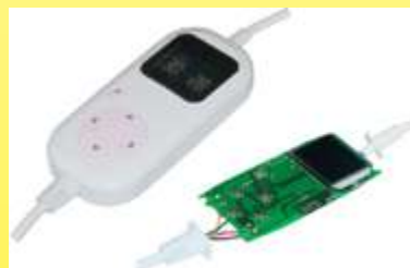
2019 Control unit for temperature-controlled heating blankets with digital display via a thermistor probe incorporated into the heated area (Ultimheat Collection)
