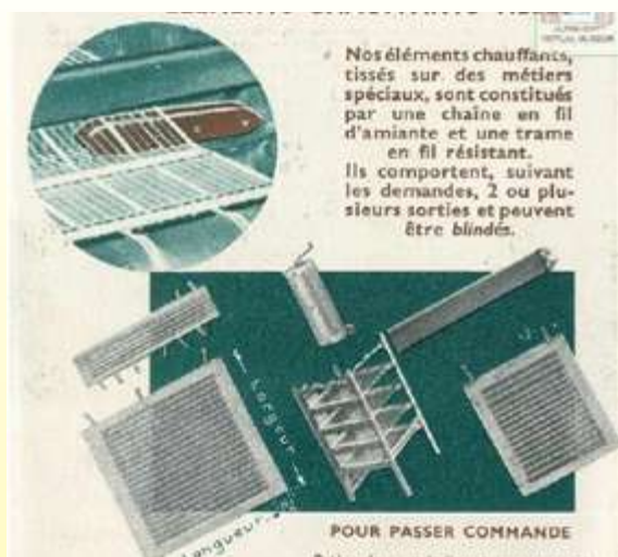
1939 Asbestos-woven elements (Noirot Catalog 1939, Ultimheat Museum)
