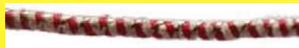
1960 ca. "Sef-regulating" heating cord from the brand Ellesert, diameter 1.2mm. The central core is a straight cotton thread surrounded by a guipure consisting of two 0.1mm diameter cotton threads wound with a 0.8mm pitch. There is then a 3 0.067mm nickel conductor guipure wound with a 0.8mm pitch in the opposite direction. This keeps the whole unit from looping (Ultimheat Collection)
