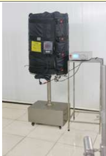
Insulation resistance measurement after IPx6 tests
