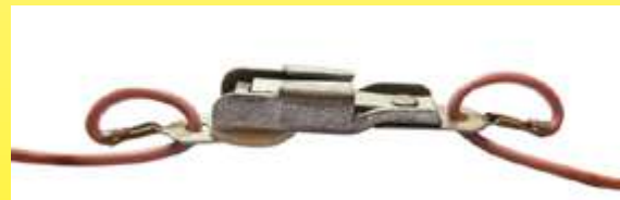
Calor slow-break heating blanket temperature limiter, calibrated at 80°C (circa 1960). Note the waterproof PVC sleeve welded on the wires and the loop made by the electrical conductors passing through a hole in each terminal- this is to eliminate tensile stresses on the wire (Ultimheat Collection)
