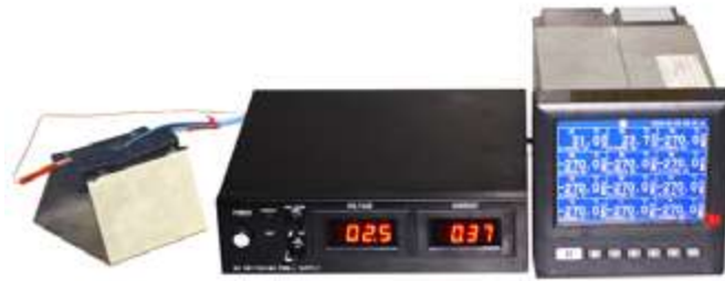
Equipment for measuring the surface temperature as a function of the surface W/cm^2 of the blanket heater or jacket heater
