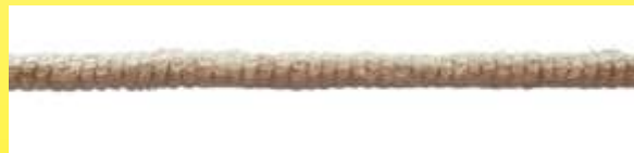
1960 ca. Calor heating cord, diameter 1.7mm, single nickel chromium heating wire, diameter 0.08mm, on a slightly twisted cotton core to prevent buckling (Ultimheat collection)
