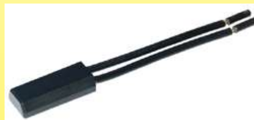
2019 Snap-off temperature limiter for heating transformer, derived from the 1966 Texas Instruments 7AM model, usable at 230V, in plastic waterproof casing. Temperature range of 5 to 8°C. Type V7AM. (Ultimheat Collection)
