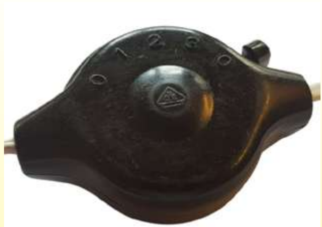
1955 ca. 5-position rotary switch similar to the Cucho model, but with snap-off switch (German manufacture LW Lohmann and Welschehold GmbH & Co. at Meinerzhagen)( Ultimheat Collection)
