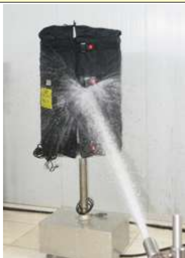
IPx6 testing of jacket heaters
